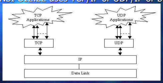
TCP is responsible for data recovery by providing a sequence number with each packet that it sends TCP requires ACK (acknowledgement) to ensure correct data is received Packet can be retransmitted if error detected ANSI C12.22 does not provide Transport Layer for non-comm-module implementations These are internal features of TCP/IP and are not visible to the ANSI C12.22 Application
